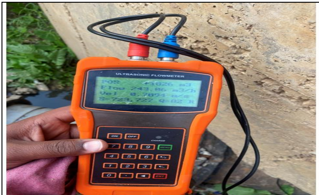
Figure :- Water Measurement on University outlet for STP
