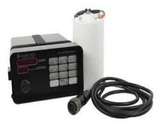
**d). Engineering Seismograph**: The department has Multichannel Analysis of Surface Wave (MASW) based 24-channel engineering seismograph (McSEIS-SX) which is used for the measurement of Vs30 and depth of bedrock in seismic microzonaton.
